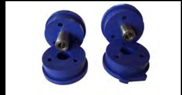
Upgraded Engine Mount Kit Part No. - Front ALS3E0277J / Rear ALS3E0278J Applications - S2 (Toyota) Exige/2-Eleven Good shift characteristics of the engine mounts require that the engine roll rate be high. Upgrading the rubber bushes to polyurethane in the front and rear mounts reduces upper engine movement by as much as 80%. Improves powertrain response, gear selection and feel dramatically. This component is track performance related and as such increases engine vibration levels felt by the occupants.
