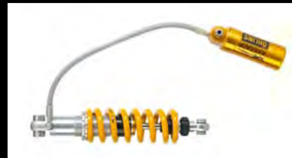
Race Specification 2-Way adjustable Ohlins Dampers* 1 Part No. - Contact Lotus Sport Available 2009 Applications - 2-Eleven A new option of Ohlins damper with revised race valving and matching stiffer spring set to suit Yokohama A048 and similar treaded tyres in full race applications, as seen on 2-Eleven GT4 Supersport.
