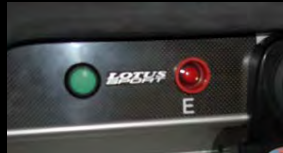
Electrically Operated Kill Switch Kit 1 Part No. - ALS3M0007K - Contact Lotus Sport Applications - Elise/Exige/2-Eleven FIA compliant kill switch allows for remote fitting in the cockpit for easier driver access, plus greater flexibility in location of external controls.
