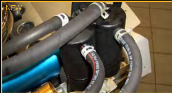
NEW Oil Catch Tank* Part No. - ALS3E0318F Applications - All S2 (Toyota) Elise/Exige/2-Eleven Fitted to the 2ZZ Engine, this Catch tank acts as a swirl pot to clean up the air flow back to the throttle providing a cleaner air for combustion.
