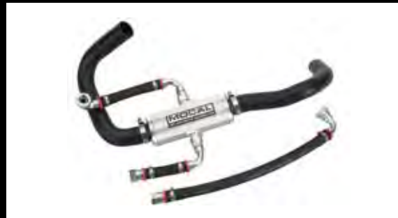
Laminova Oil System* Part No. - DLS3E0259F Applications - All S2 (Toyota) Elise/Exige/2-Eleven Replaces the existing twin front mounted air to oil coolers with a water to oil high thermal efficiency heat exchanger. Offers maximised heat dissipation for minimum pressure drop on each media side, when used with the triple pass front radiator.
