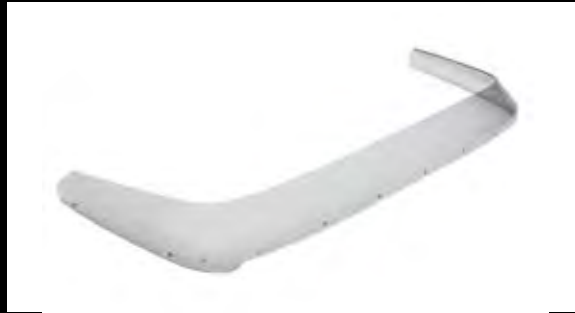
Lotus Sport 2-Eleven High Windscreen Part No. - A127B0161F Application - 2-Eleven A 1" taller windscreen to reduce 'buffetting' experienced by taller drivers.
