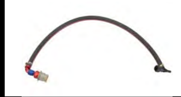
Fuel Drain System* Part No. - ALS3L0072F Applications - All S2 (Toyota) Elise/Exige/2-Eleven Mandatory FIA requirement for racing. Allows the fuel cell to be drained easily and quickly.
