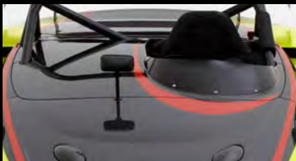
Carbon Fibre Rigid Tonneau Cover* Part no. - TBA Applications - 2-Eleven High quality 'pre-preg' carbon fibre rigid tonneau cover. Converts vehicle to a single seater with wrap-around 'aero' screen. Can be finished to customers request depending on requirements. Please call to discuss. Strictly for track use only. Natural finish carbon fibre may deteriorate in appearance over time if exposed to extreme weather conditions or sunlight.
