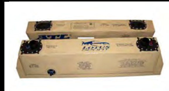
100L ATL Fuel Cell* - Special Order Applications - Exige 100 litre competition specification bag tank. Allows the fuel supply system to function under the most demanding of race conditions while complying with all FIA requirements. Specialist fittings required. Please call for further information regarding this part. Note: Part has a 5 year maximum service life.
