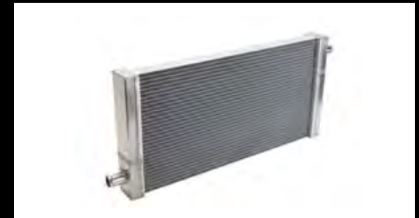
Triple Bypass Radiator Part No. - ALS1K0006F (S1 & S2 K-series) ALS3K0034f (S2 (Toyota) Elise/Exige/2-Eleven) Forces the water to pass through the radiator three times instead of the normal single pass, this can vastly reduce the engine coolant temperatures.
